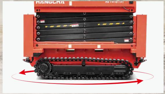
The steering proportional deceleration and electronic differential function can make the machine pivot steering.
