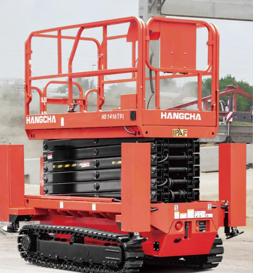
The scissor cylinder adopts proportional descent control, the moving speed changes gradually with the tilt angle of the operating joystick, and the descent is smooth and comfortable.
